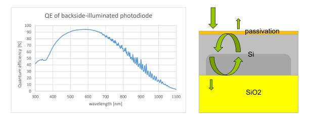
The major weak point is the 'etaloning' or interference patterns in the near infrared region. For longer wavelengths, the absorption length of silicon increases and the silicon layer begins to behave as an optical cavity, causing interference.
