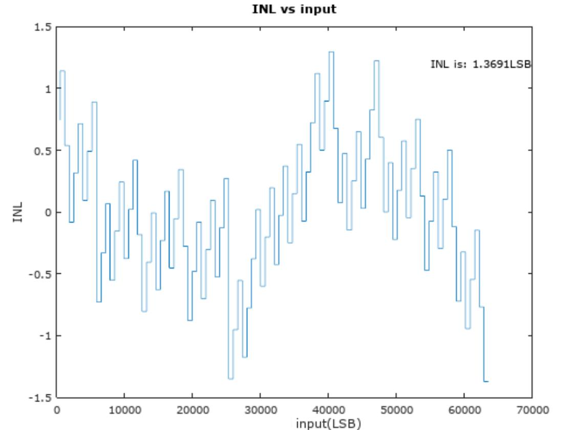
Differential input with PGA gain: 0dB
