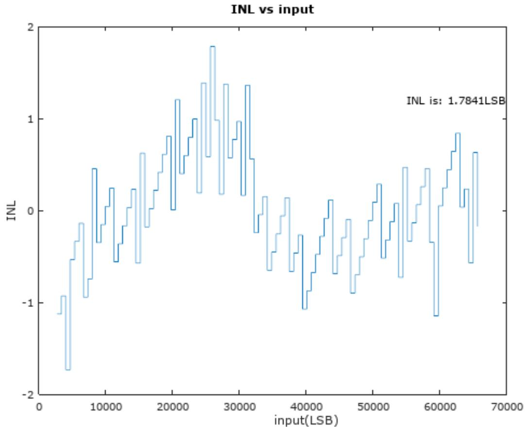
Single ended input with PGA gain: 0dB
