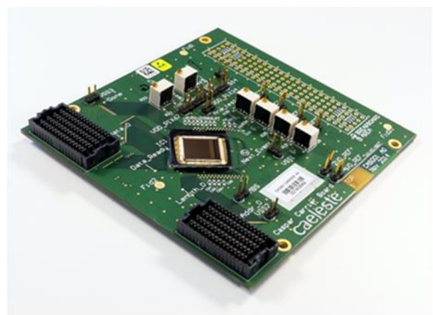
Figure 7 picture of layout and the IC on the CoB test board
