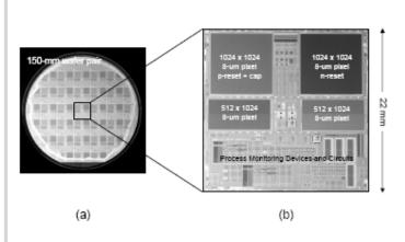
19.6.4: (a) Completed 3D integrated wafer pair, (b) Die photomicrograph
