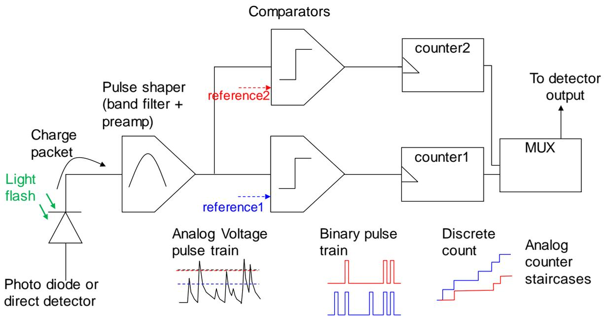
Figure 3 The 2-Color X-photon counting pixel circuit topology
