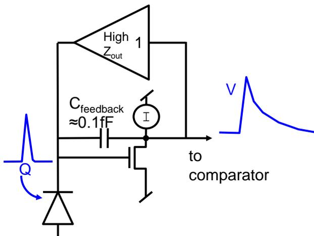
Figure 5 Pulse shaper circuit topology
