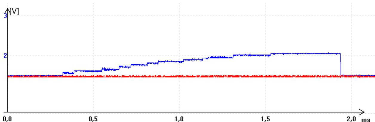
Figure 8 Real time trace of the counter staircase of a QX2010 pixel as direct detector (i.e. without scintillator). X-ray source at 1.5m distance; 100kVp, 70mA.
