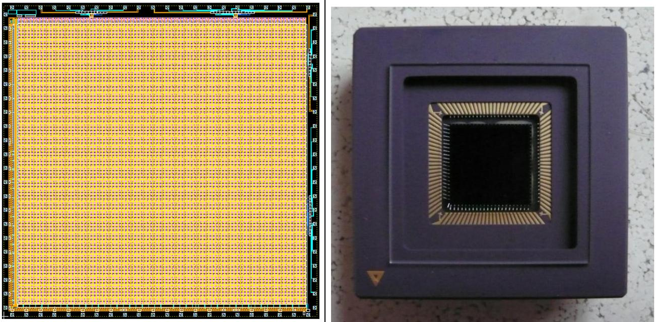
Figure 2 Layout drawing and picture of the QX2010 92x90 pixel color x-ray photon counting demonstrator.
