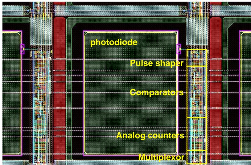
Figure 4 Layout view of the QX2010 pixel.
