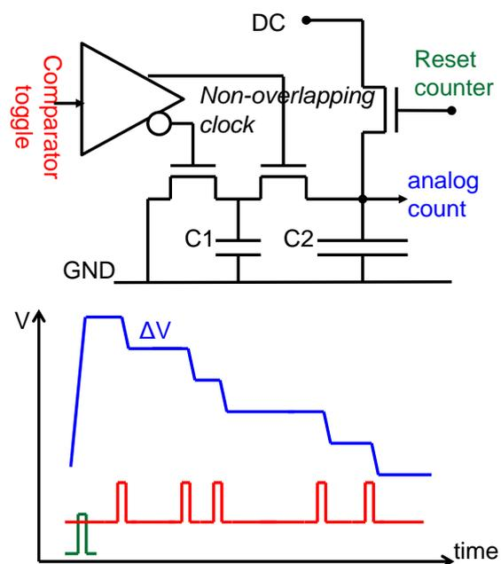
Figure 6 Analog counter and its key signal traces.
