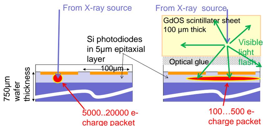
Figure 1 Direct (left) vs indirect (right) X-photon detection in the present device.
