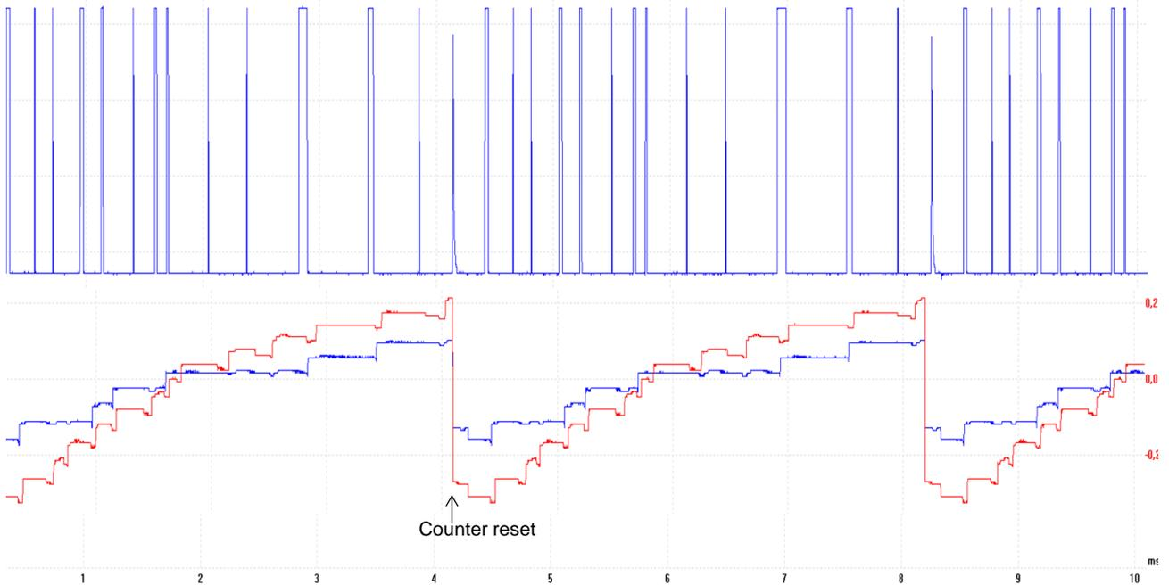
Figure 7 Real time observation of counting staircase for light pulses pattern generated with a LED. Upper trace: LED pulse pattern, where a wide pulse generates a larger charge packet. Lower traces red/blue: counter staircases for the two channels (trace acquired AC-coupled). The red channel counts every LED pulse. The blue channel counts only the wider LED pulses.
